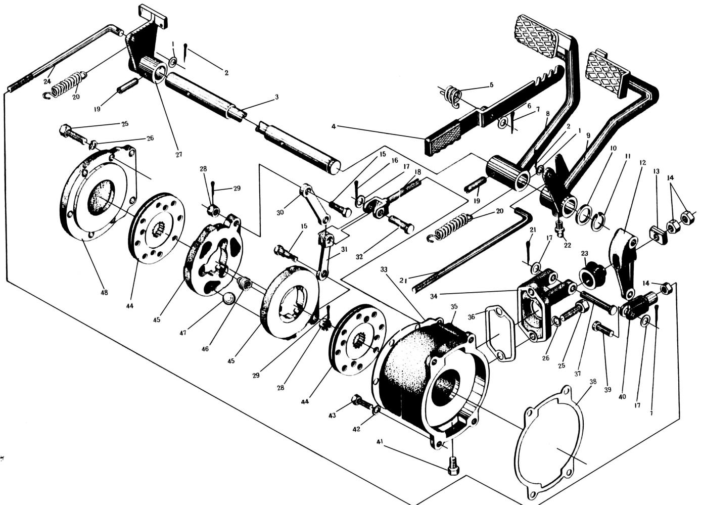
Fig. 12 Brake And Operation Mechanism II
